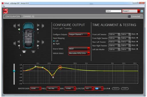
**Figure 12 Master Equalization**
